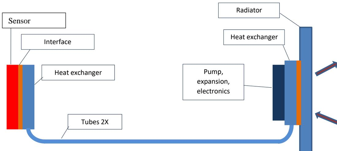
**Figure 2. System overview.** The developed thermal regulation system with sensor and radiator added for clarity. The emulated sensor is simply a heater while the radiator temperature is controlled externally to emulate a LEO orbital variation in absorbed heat flux on the radiator.
