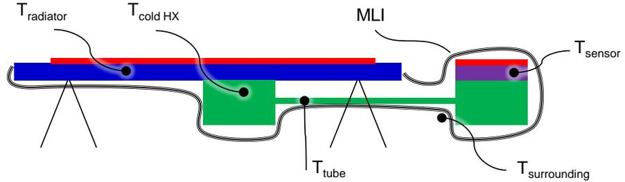
**Figure 4. Lab bench test.** The system was suspended on insulating legs and wrapped in MLI prior to measurements. The thermocouple positions are indicated.
