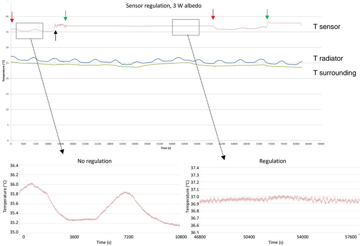
**Figure 6. Heat flux perturbation and regulation.** An earth albedo heat flux variation is simulated on the radiator. This perturbation is decreased using PID control of the pump (PWM). Red and green arrows indicate off and on for the regulation while the black arrows shows the PID auto-tune.
