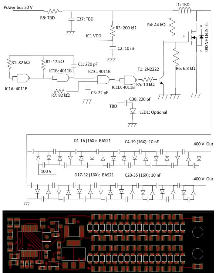
**Figure 8. Electronics schematic above and PCB layout below**
