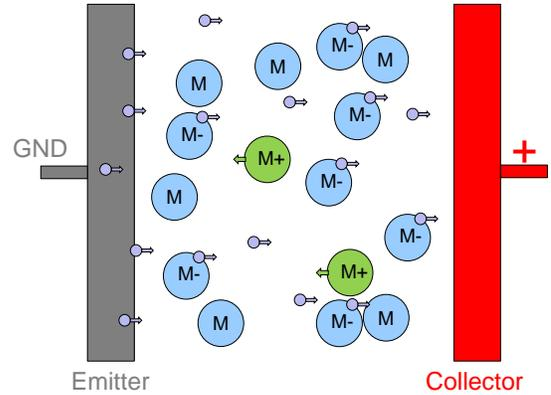
**Figure 1. Ion drag pumping.** A flow between emitter and collector is created by the ion drag from accelerating ions. Using perforated electrodes, a net flow to the right is generated.
