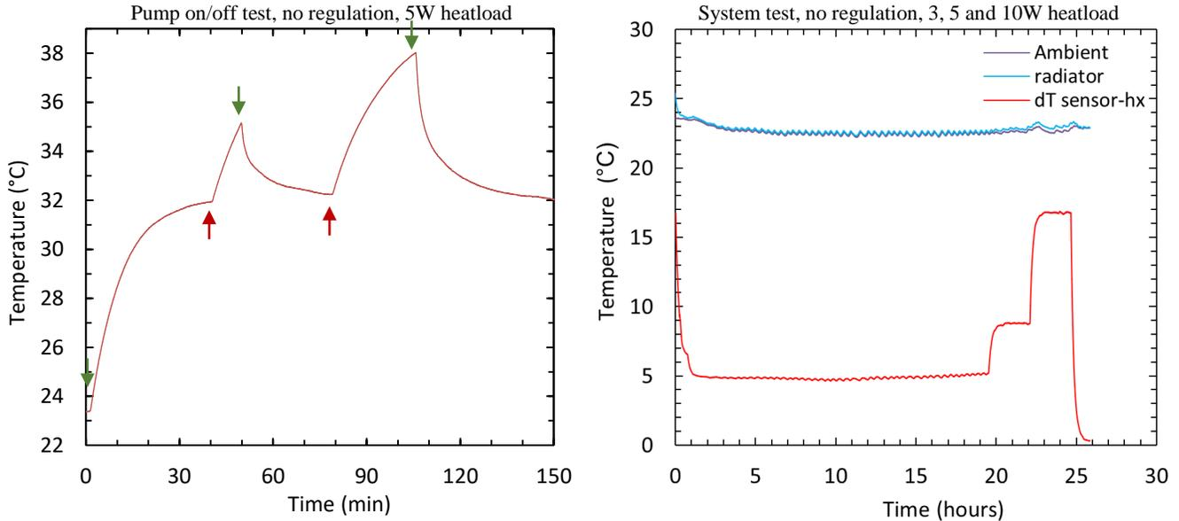
**Figure 5. Left: Pump on/off test.** The pump is cycled on (green arrow) / off (red arrow) with a heat load of 5 W and a room temperature of 23.5 °C. **Right:** 3, 5 and 10 W of heater power with the pump always on. Ripple comes from room airconditioning. The red line corresponds to the temperature difference between the sensor and the cold heat exchanger.
