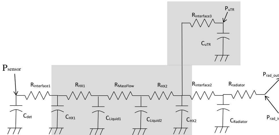
**Figure 7. Reduced thermal mathematical model.** The developed system is within the marked area.
