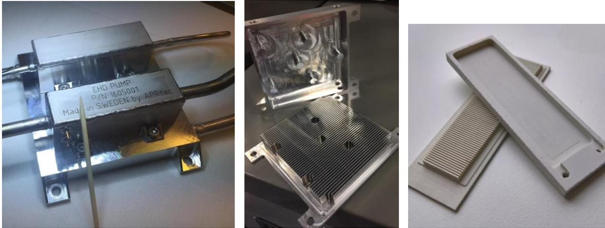
**Figure 3. Left: Cold side heat exchanger assembly.** The cold side heat exchanger carries the liquid expansion chamber (top) and EHD pump (bottom). A tooth pick has been added for scale. **Center: Cold aluminium heat exchanger before assembly.** **Right: Shapal heat exchanger before assembly.**
